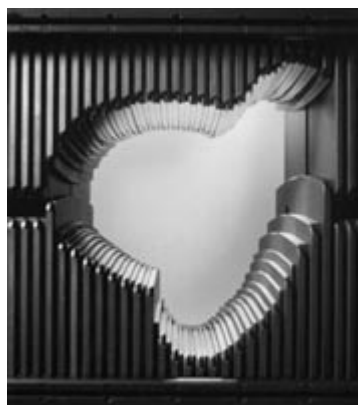
Figure 2: Leaf pairs of multileaf collimator. Radiation will pass through the open area.
